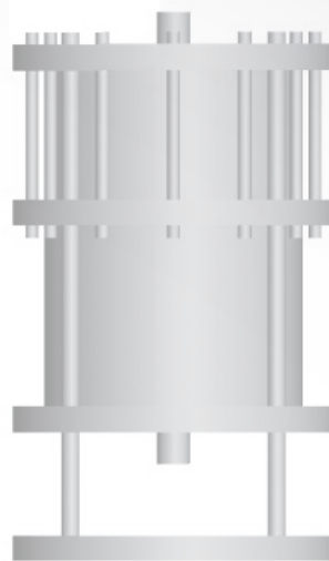
Pic. 1: Chromatographic columns have a limited loading capacity for polishing and virus capture. Furthermore, they are large and have a high investment cost.
