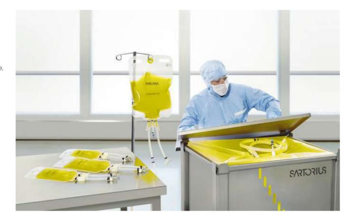
By combining speed and efficiency to deliver high-performance mixing during powder dissolution with a levitating impeller to preserve the drug during low shear blending applications, the Flexsafe® Pro Mixer can accommodate a wide range of mixing operations
