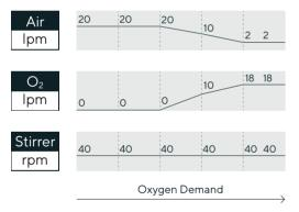
Constant gas flow decreases the flow of air and simultaneously increases oxygen gas
