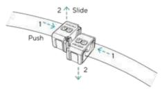
4. Disconnect the Clipster® Aseptic Disconnector.
