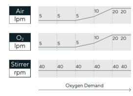
Constant gas ratio, where both air and oxygen % are increased at the same rate
