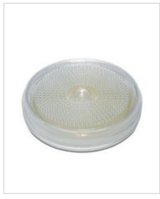
Sartorius has developed a new system for sampling airborne microorganisms that allows impaction onto culture media plates, where the plates function directly as collection heads.
