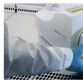
This new method uses the AirPort MD8 air sampler to pump the air stream.
